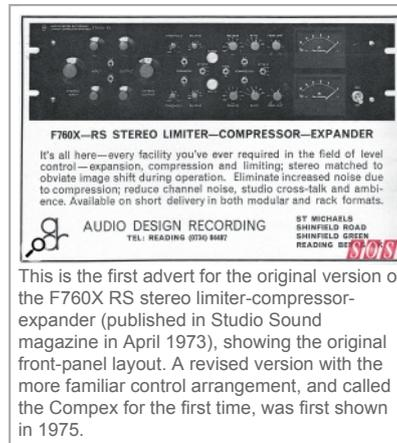
This is the first advert for the original version of the F760X RS stereo limiter-compressor-expander (published in Studio Sound magazine in April 1973), showing the original front-panel layout. A revised version with the more familiar control arrangement, and called the Compex for the first time, was first shown in 1975.
