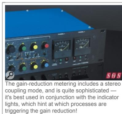
The gain-reduction metering includes a stereo coupling mode, and is quite sophisticated — it's best used in conjunction with the indicator lights, which hint at which processes are triggering the gain reduction!
