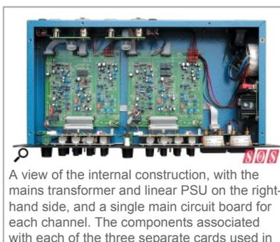
A view of the internal construction, with the mains transformer and linear PSU on the right-hand side, and a single main circuit board for each channel. The components associated with each of the three separate cards used in
